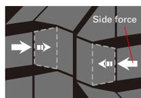
As the tire comes into contact with the ground, the circumferential groove shifts as it closes, thereby lessening the force from the side.
